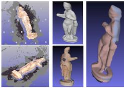
**Fig. 3.** Processing 3D scans: Raw 3D scans (left column), scans after noise removal (centre column) and a resulting model (right column)
